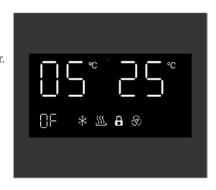
The temperature display will show the set temperature when the Wine Cooler control panel is unlocked and selected to be reset, and show the actual temperature when the control panel is locked.
